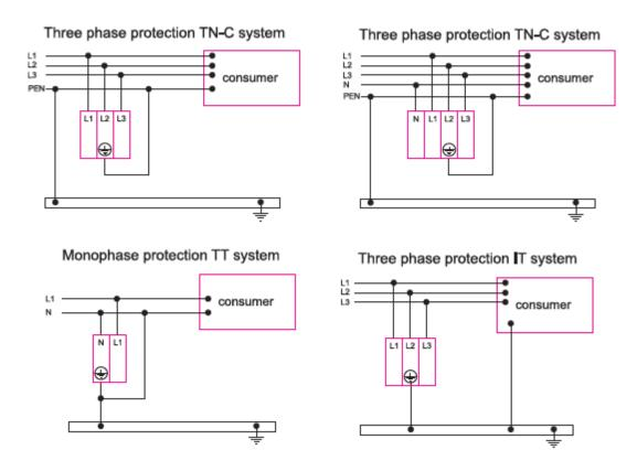
The surge arrester selection is made according to the overload risk level or atmosphere activity, named B, C or D (from high to low risk level).
